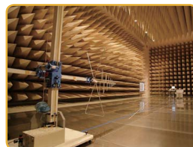
EMC testing facility
